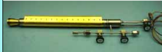
1 stage laboratory-scale (10-50 bar, 60 L/h H 2 ) MH compressor ( IFE, Norway )
