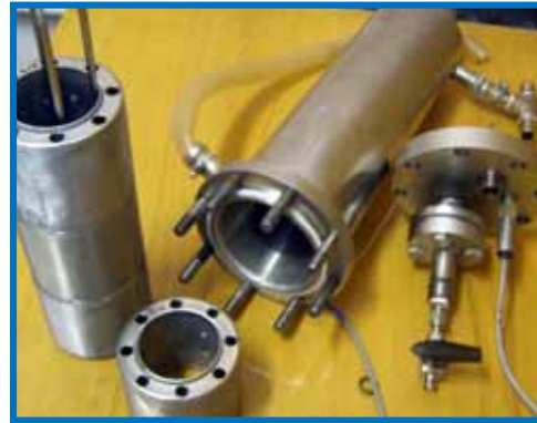
PXO-2: shell and tube type reactor with outer and inner cooling of hydride bed inside tubular cartridges
