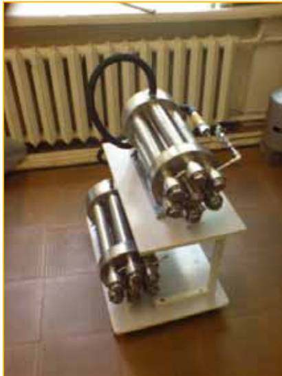
PXO-3: shell and tube type reactor with outer and inner cooling of hydride bed inside tubular cartridges
