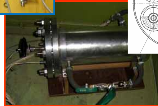
PXO-2: shell and tube type reactor with outer and inner cooling of hydride bed inside tubular cartridges
